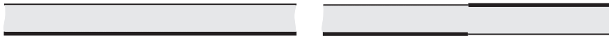
Figure 1: Planar strips with untwisted (left) and twisted (right) boundary conditions; the thick and thin lines correspond to Dirichlet and Neumann boundary conditions, respectively.
