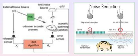
Acoustic noise reduction Active versus passive controllers.
