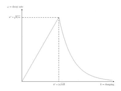
We observe here the classical overdamping phenomenon. Contradicting a first intuition it is not true that the decay rate increases when the value of the damping parameter k increases.
