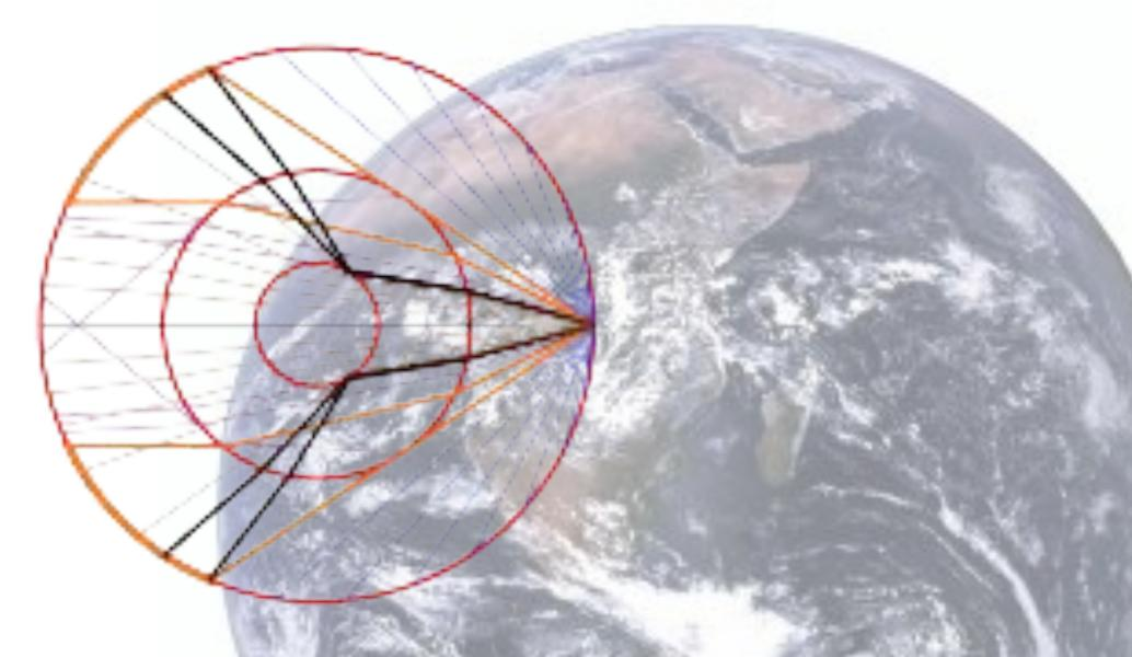
The signal travels faster in the inner core. So some rays cannot enter and are reflected. They are detected in the forbidden region of the orange arcs.
