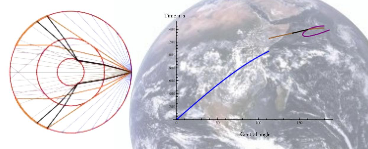
The travel times do not allow to distinguish between the black rays reflected on the inner core and the brown rays that enter and exit the inner core.
