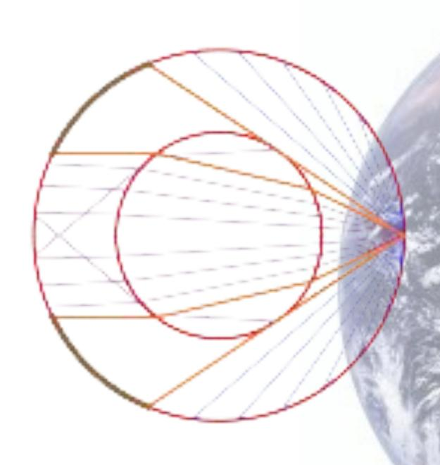
We see that no signals can be detected along the two brown arcs located between 112 degrees and 154 degrees.
