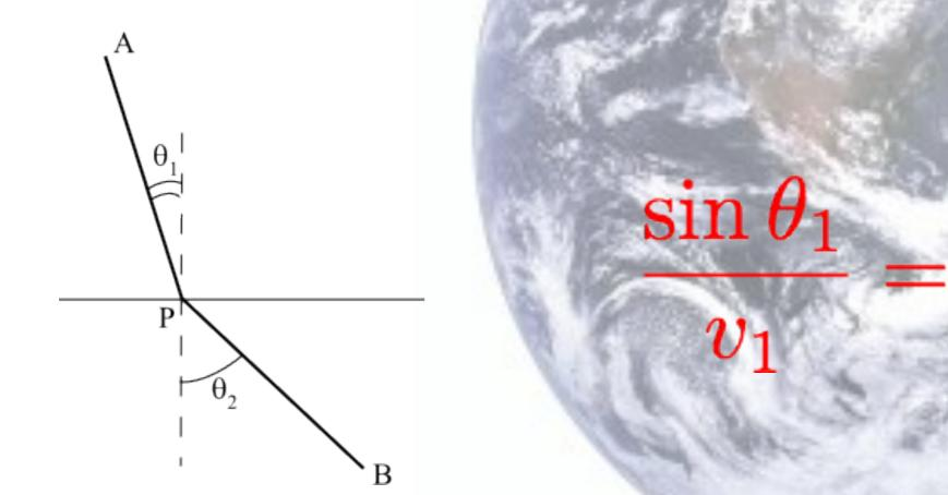
This is what occurs when leaving the mantle and entering the core in which the signal slows down.
