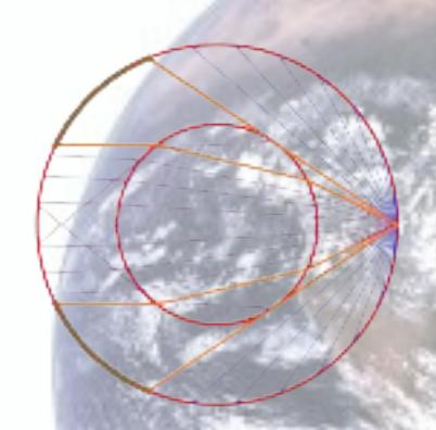
A model explaining the anomalies and the registered travel times for these signals is that the core is divided in two parts: the inner core and the outer core.
